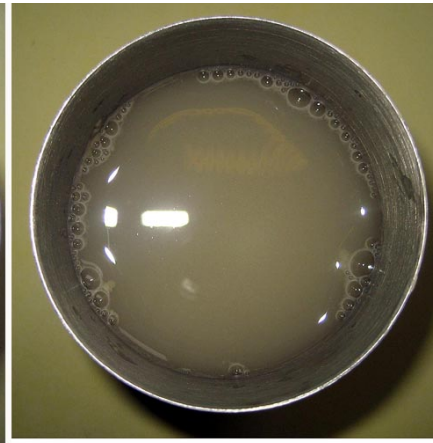
5 minutes later most of the Bentonite clay has dissolved in warm water with some stirring.
