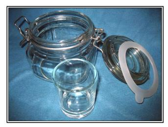
500 ml capacity clamp-lid glass **receiver** container, silicone lid-to-jar **gasket**, and 90 ml capacity **reactor** glass candle holder. **Reactor** is 2" (5 cm) diameter, 2.5" (6.35 cm) tall.
